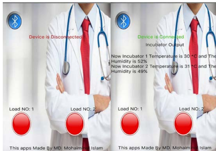
Figure 6: Projected Andriod Based Application for Infant Incubator showing Device connectivity
