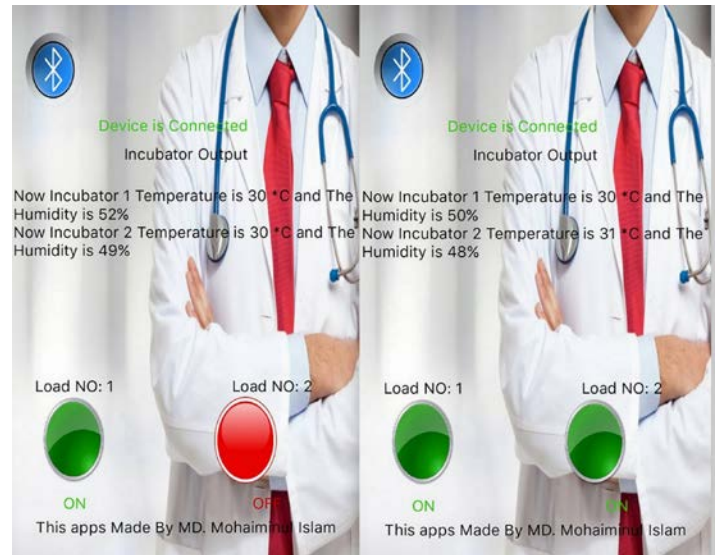
Figure 6: Projected Andriod Based Application for Infant Incubator showing temperature and humidity of the incubators.
